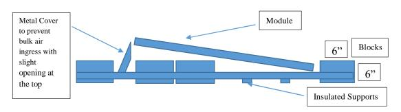
Each block should be of 25 Kg weight & should be cubical shaped reinforced concrete with dimensions of 1.5 feet (length)\*6 inch (breadth)\*6 inch (height) with a cut-out of 100 mm\*60
