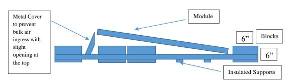
Each block should be of 25 Kg weight & should be cubical shaped reinforced concrete with dimensions of 1.5 feet (length)\*6 inch (breadth)\*6 inch (height) with a cut-out of 100 mm\*60 mm across the breadth
